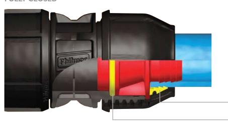
Split collet bites into the pipe providing end load resistance
